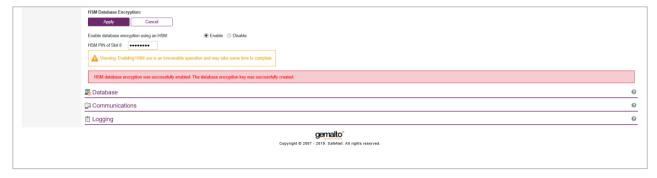
**NOTE:** If the AES key with Label: HSM\_KEY\_AES\_ENCRYPTION\_VER\_13 exists in Luna HSM partition, then it will use the existing key. If there is no key with this label, it will generate a new key.
