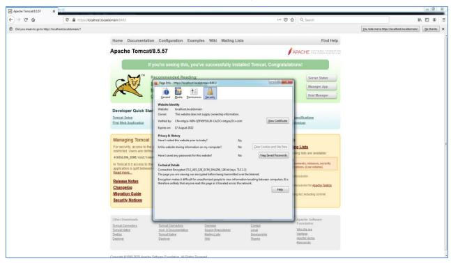
This completes the Apache Tomcat integration with Luna HSM and SSL certificate private key is secured on HSM partition. The SSL page will be accessible only if HSM partition is accessible and available to Apache Tomcat Server
