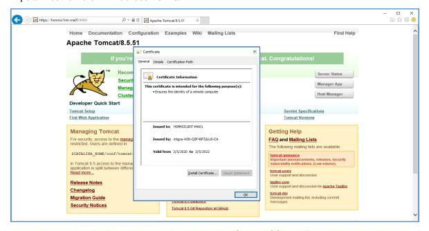
This completes the Apache Tomcat integration with Luna HSM and SSL certificate private key is secured on HSM partition. The SSL page will be accessible only if HSM partition is accessible and available to Apache Tomcat Server.
