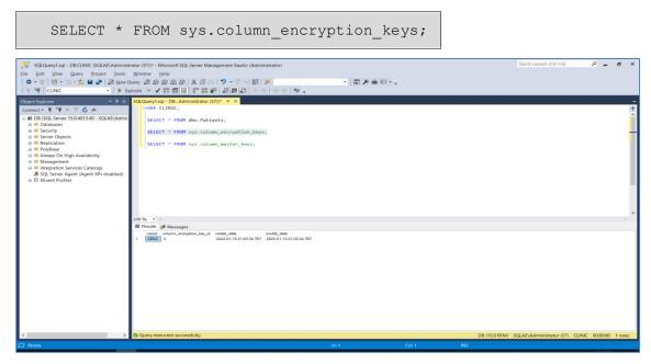
The rotation of column encryption key is completed successfully and you can view the encrypted columns (encrypted using new CEK) using <u>View Always Encrypted Data</u>.
