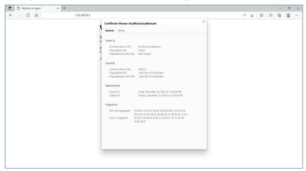
This completes the NGINX integration with Luna HSM. The SSL private key of NGINX server is now safe and secured on Luna HSM partition. The SSL page will be displayed only if the HSM partition is accessible and available to the NGINX Server.
