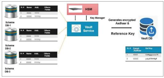
In the above diagram, Thales Luna HSM used for storing digital signature certificate for encrypting Aadhaar numbers.
