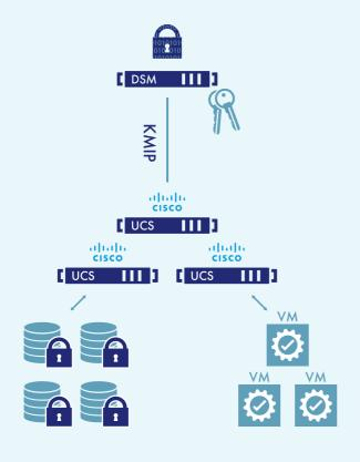
Vormetric DSM protects and manages the cryptographic keys used by Cisco UCS within a FIPS 140-2 Level 3 appliance.
