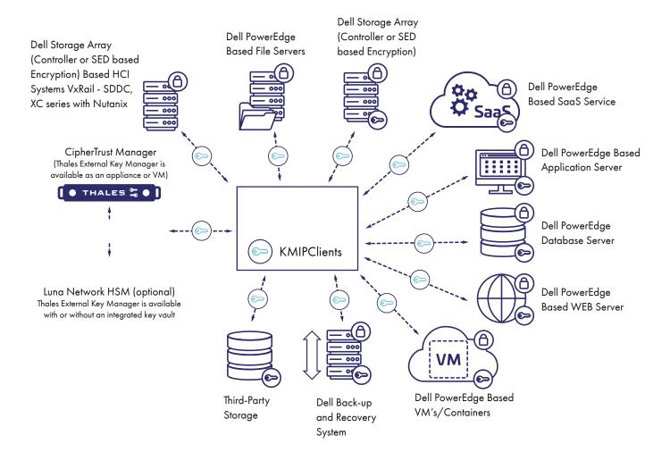
Offered as part of Dell OpenManage Secure Enterprise Key Manager, Thales CipherTrust Manager simplifies and centralizes encryption key policies and management, and helps meet global compliance, security, and privacy standards.
